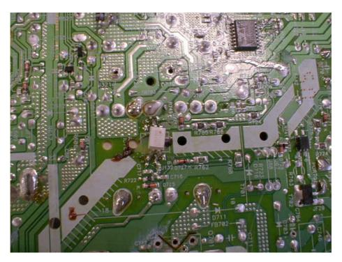
Please note the positioning of the opto couplers in the case of IC705 (power) above and the data opto couplers (IC703 and IC704)
